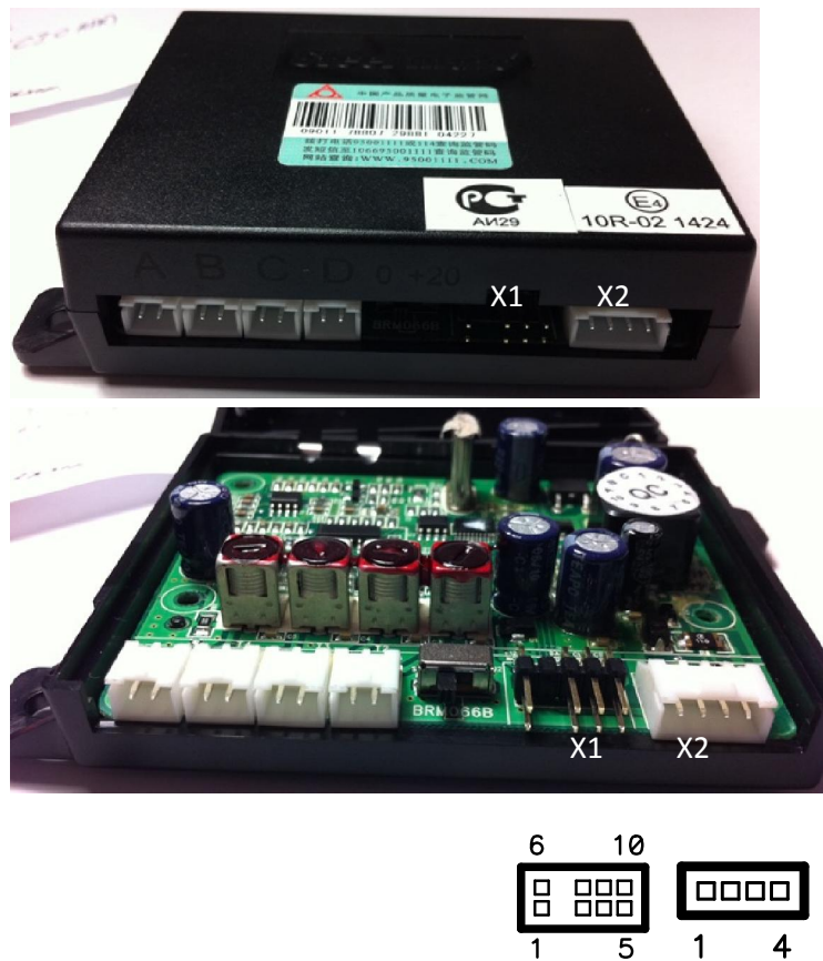
Fig 2 Design and pinout of external control unit PTS400M6
