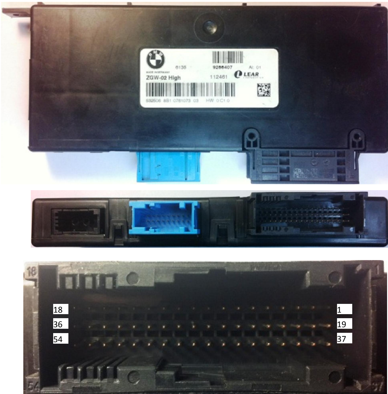
Fig 5 ZGW design and pinout
